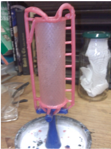
Wax vessel ready for casting – It was important it was made this way so when cast in silver it had no solder seams
